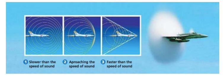
When the plane travels almost as fast as the speed of sound, the sound waves pile up in front of the plane. This pile-up is the "sound barrier." As the plane flies faster than the speed of sound, it moves through the barrier. A shock wave forms as the sound waves overlap. The shock wave releases a huge amount of energy. People nearby hear a loud noise called a **sonic boom** when the shock wave passes by them.
